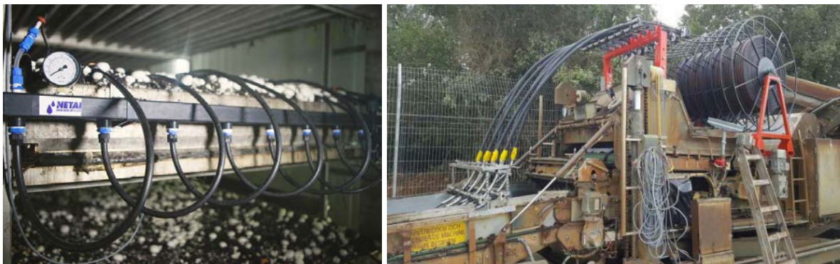
Figure 32. The Netafim "Mushroom Master" drip irrigation system (left) and the insertion unit on a Thilot head filler. From Raz et al., 2016.
