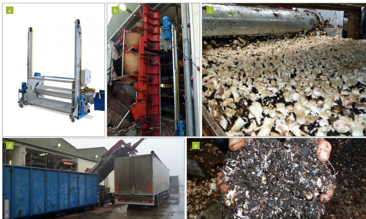
Figure 3. The Mush Comb unit (a) is used to separate the casing from compost during room unloading. The separator is used with a multi-arm emptying machine (b) as the crop is removed after final harvest (c). Conveyors take compost into the waiting trailer, while casing is diverted to a container at one side (d). The separated casing soil (e) and compost can then be recycled or used for other purposes.
