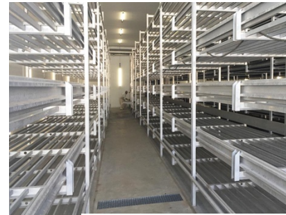
Metal shelving is easier to clean and more energy efficient than wooden trays
