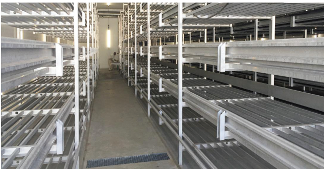
Figure 3. Galvanised belt and shelf systems allow more efficient cook-out than older wooden tray systems
