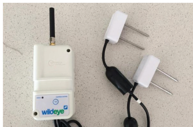
Figure 5. Wildeye TDR soil moisture sensors and communications unit
