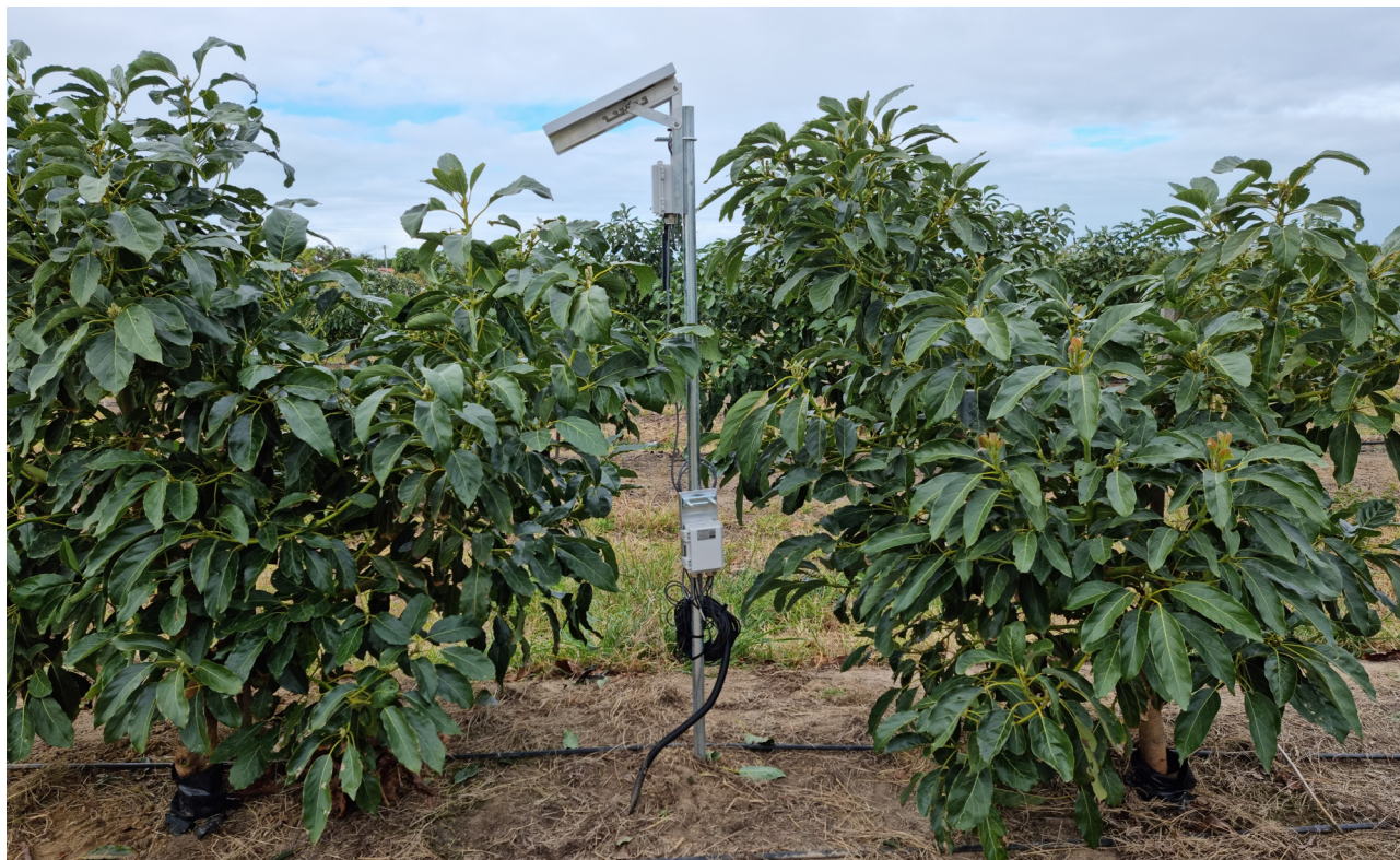
Communications node with dendrometer and soil moisture sensors with a dendrometer
