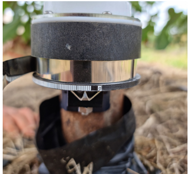
Band dendrometer installed on avocado tree
