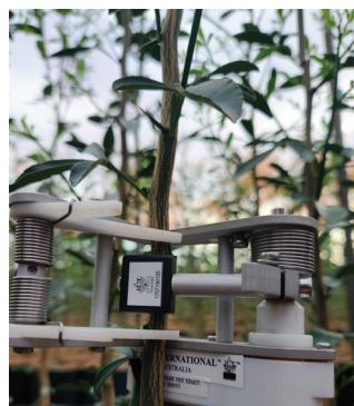
Pivoting stem dendrometer installed on a young citrus tree
