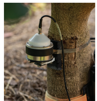
Band dendrometer installed on an avocado tree.
