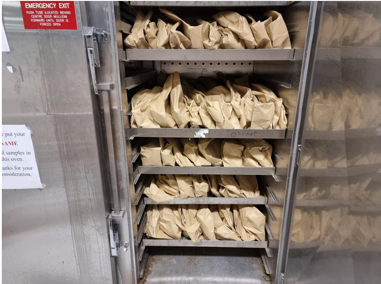
Figure 22: Lettuce heads were individually bagged for drying in a fan-forced plant dehydrator.
