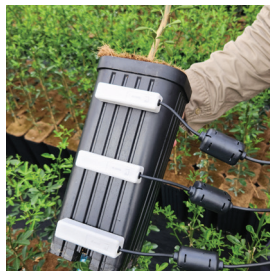
TDR moisture probes inserted into a plastic container
