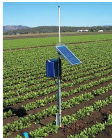
Figure 3. The photograph on the left shows a C-Probe ® soil moisture system installed in the field and the photograph on the right, shows two EnviroScan ® soil sensors which are used to detect soil moisture. The sensors are enclosed in a PVC tube to protect the electronics from soil and water.
