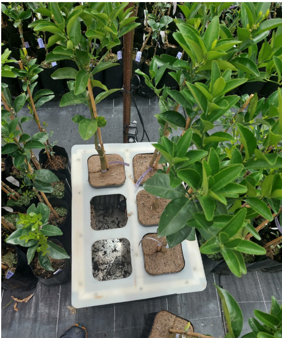
Figure 10. Container scales which are used to estimate moisture in potting media.
