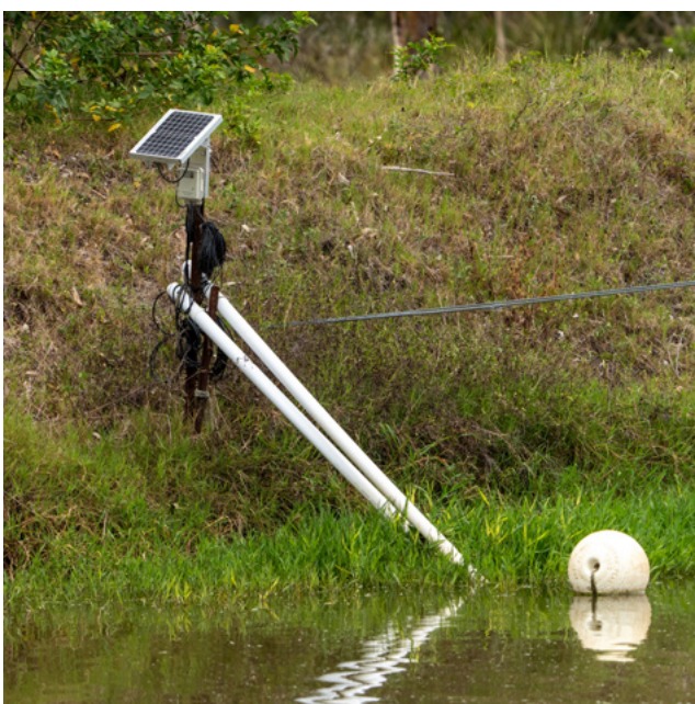
Figure 27. Dam monitoring system with buoy to keep sensors at a constant depth.
