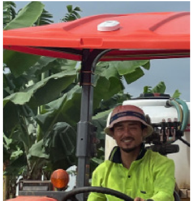
Figure 23. Tractor with a GPS tracker installed on the roof. Data is transmitted every five minutes. The GPS tracker is connected to the vehicle power supply.
