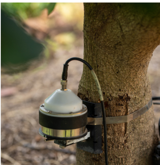
Figure 12. Band dendrometer installed on an avocado tree.
