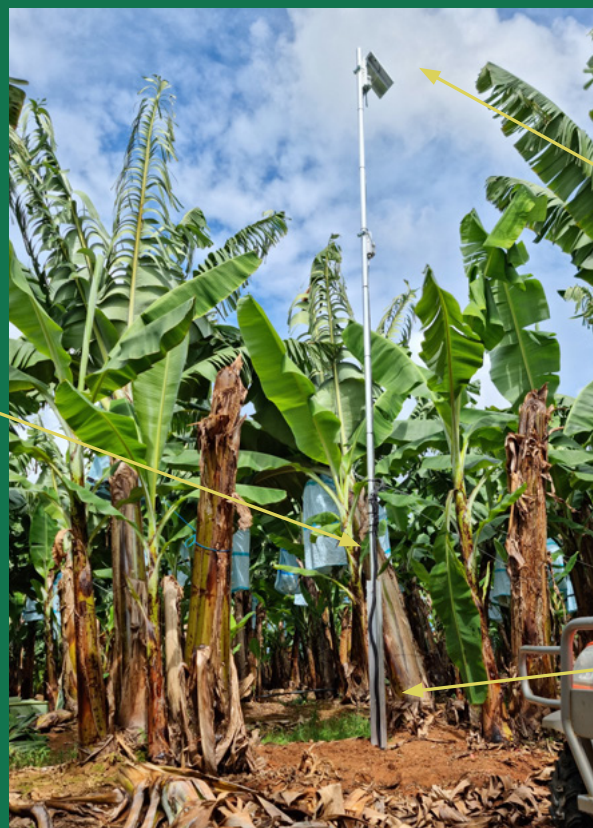
Figure 2. Best practice for solar powered sensor installation in banana or perennial crop.
