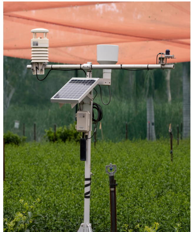
Figure 16. Weather station installed on a portable tripod at a production nursery. Temperature, wind and humidity sensor (left), tipping bucket rain gauge (center) and solar radiation sensor (right) are shown. This weather station monitors the micro-climate within the net house.
