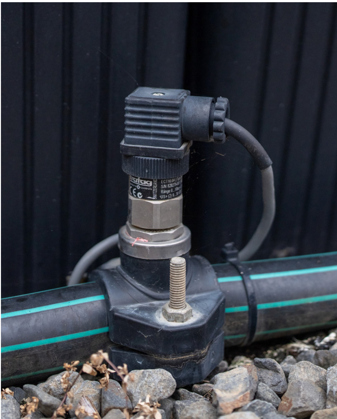
Figure 20. Irrigation pressure transducer installed on 40mm Polyethylene tube irrigation line at a production nursery.
