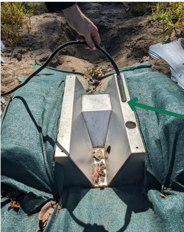
Figure 19. Submersible pressure transducer for accurately measuring water levels. Source: Keller Instruments.
