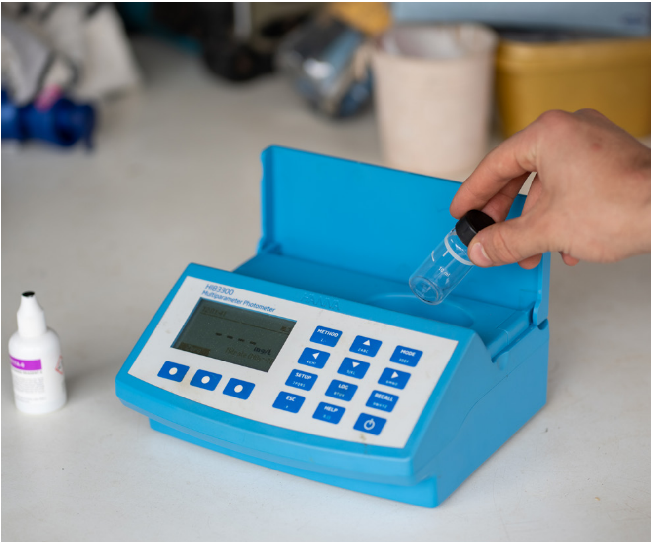
Figure 39. Desktop photometer used to measure nitrate, phosphate, chlorine and alkalinity of water samples. Results are used for EcoHort reporting.
