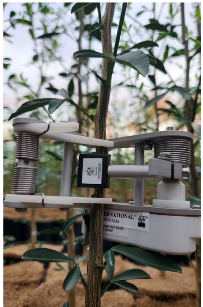
Figure 13. Pivoting stem dendrometer installed on a young citrus tree.
