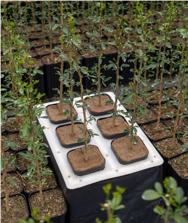
Figure 8. Weight based potting media moisture monitoring system.
